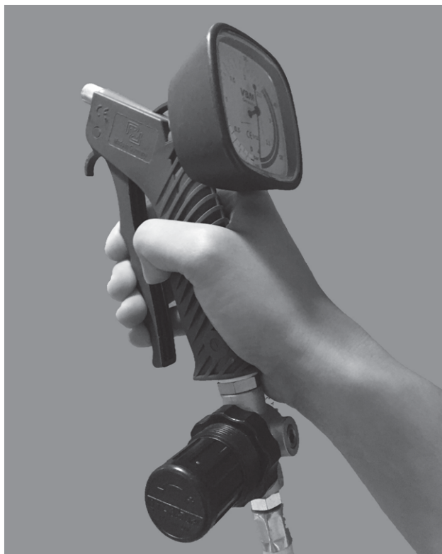
Figure 4: VBM ® Manujet III for jet ventilation having a pressure regulator and a pressure gauge
